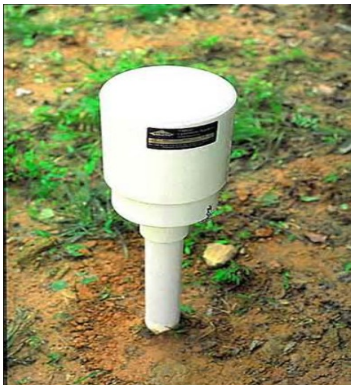
Slika 8. Lizimetar (izvor: http://www.digopaul.com/cn/english-word/lysimeter.html )
