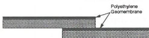
D. Bentonite-Polyethylene Composite GCL with Cap Strip
