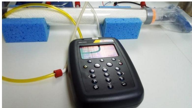
Slika 8 Geotech GA5000 Gas Analyser
