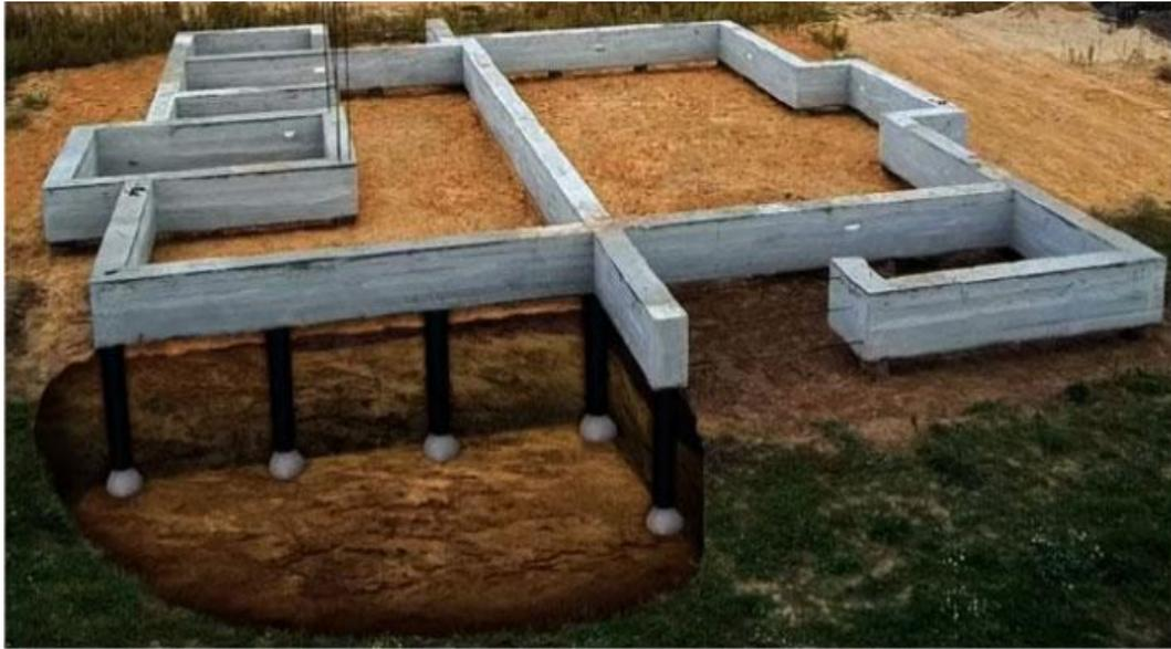
**Slika 8.** Drveni piloti (<https://hourstrong.com/pile-temelj-drvenih-pilota/>)
