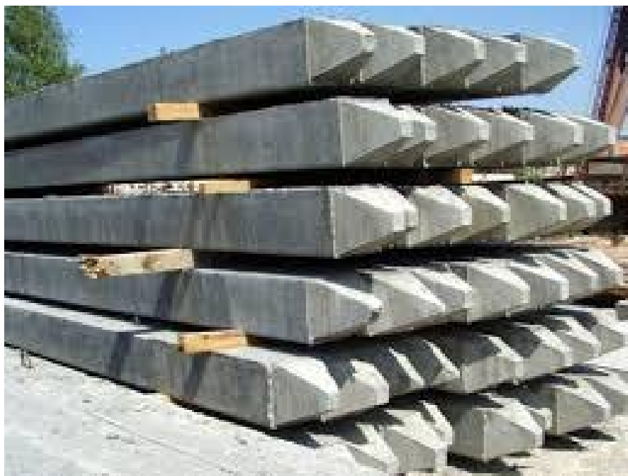
Slika 11. Betonski piloti ( https://www.structuralguide.com/concrete-piles/ )
