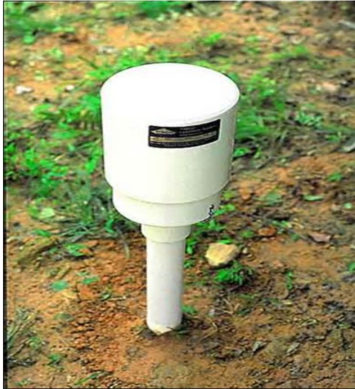
Slika 8. Lizimetar (izvor: http://www.digopaul.com/cn/english-word/lysimeter.html )
