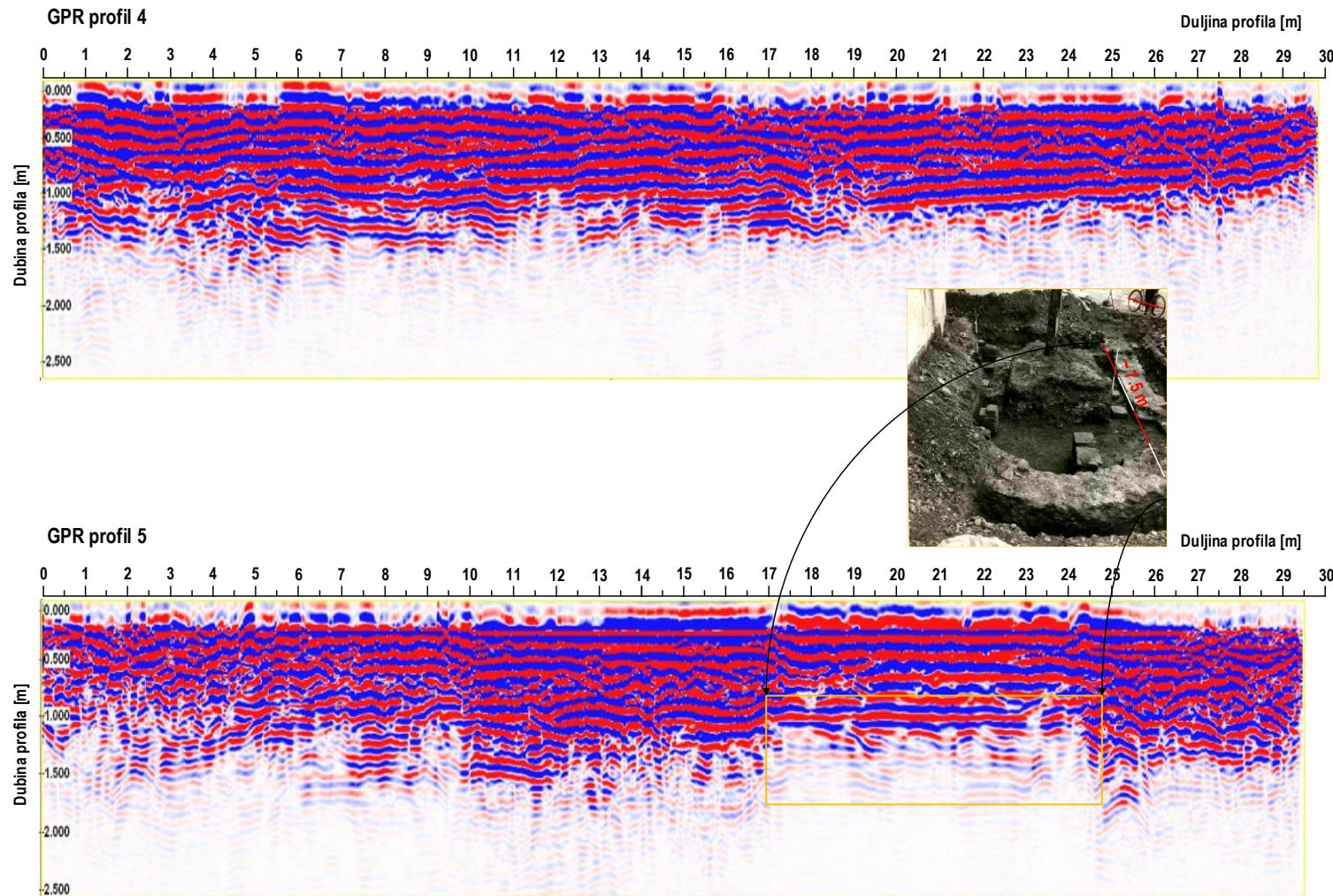
Slika 7. Radargrami GPR profila 4 i 5.
