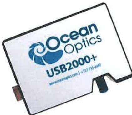
*Slika 8 Spektrometar Ocean Optics USB2000+ [32]*
