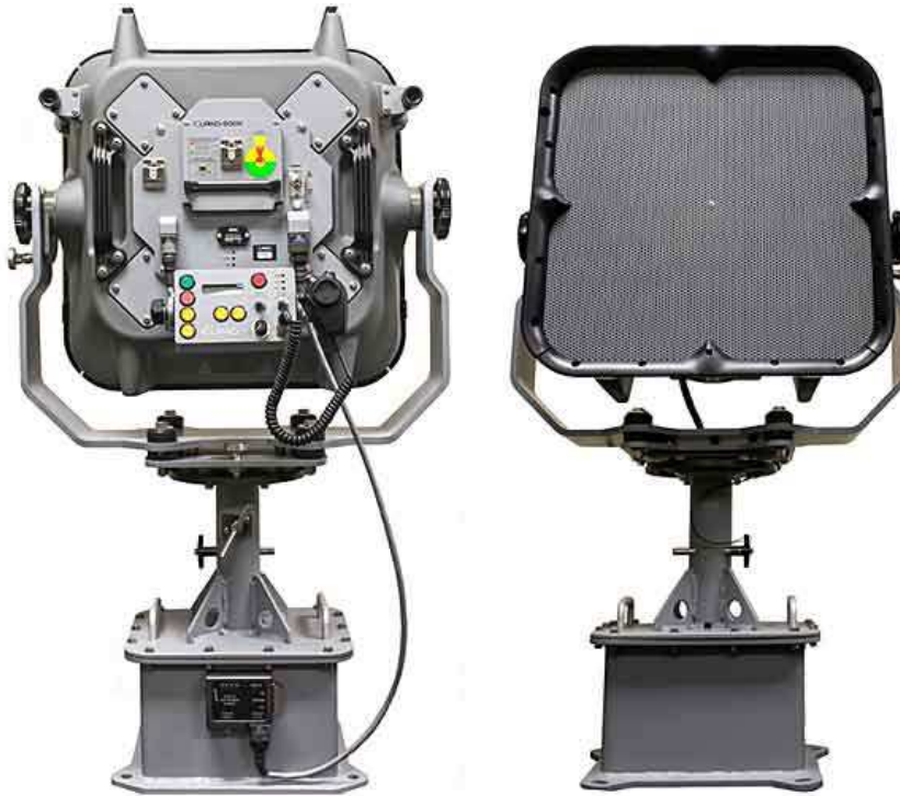
Slika 25. LRAD (long range acoustic device)
