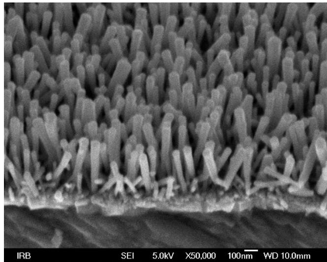
Slika 17  $\text{TiO}_2$  nanocjevčice
