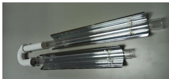
Figure 11. The setup for the CPC reactor (2 quartz tubes connected with a PTFE U-tube placed in a compound parabolic mirror)
