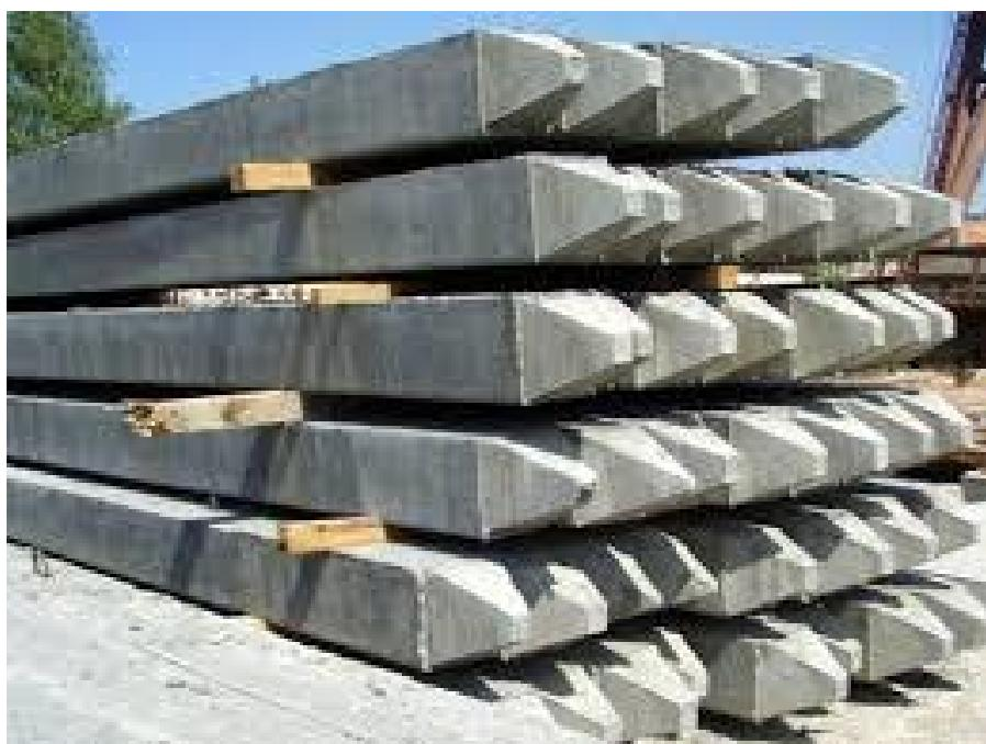
**Slika 11.** Betonski piloti (<https://www.structuralguide.com/concrete-piles/>)
