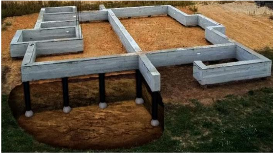
Slika 8. Drveni piloti ( https://hourstrong.com/pile-temelj-drvenih-pilota/ )
